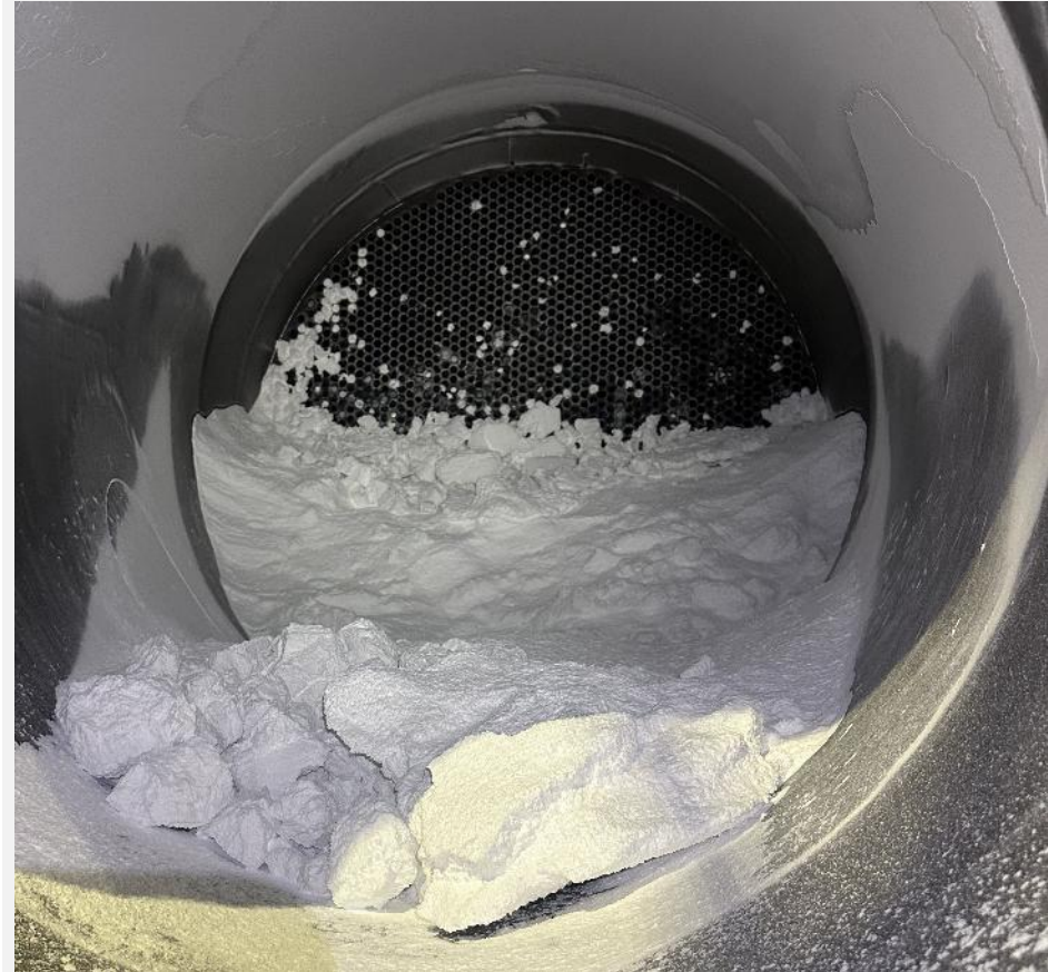
Example of polymer buildup at HE head
