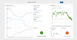
To further optimize operations, engineers also created a new tag that calculated the heat transfer coefficient of the evaporator just after the extractor. When the heat transfer rate dropped, engineers knew it was time for the process to be cleaned.
